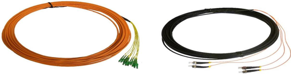
The universal breakout cable consists of 4 or more fiber optic cables. Each single cable has a 900µm coating. A layer of aramid yarn is placed around the core. The cable is completed with a outer sheath made of LSOH.
